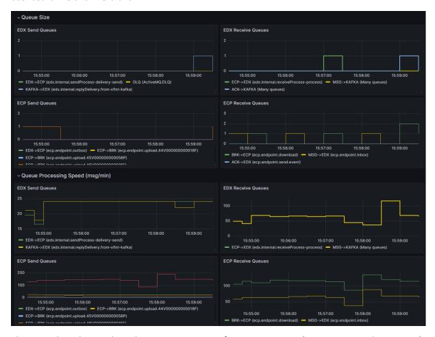
The 4 panels at the top show the queue-size-metric for various queues (EDX vs ECP, Send vs Receive). The 4 panels at the bottoms shows the dequeue-count-metric, where we measure the change in the count pr min. The same division between ECP/EDX and Send/Receive is applied.
